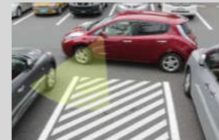
Detect parking space and park automatically
